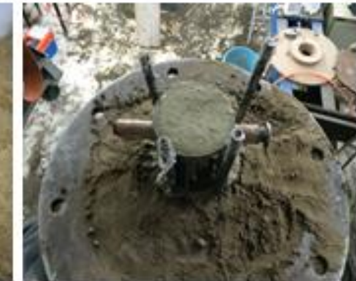
Shaft post-grouted precast-in-place pile
