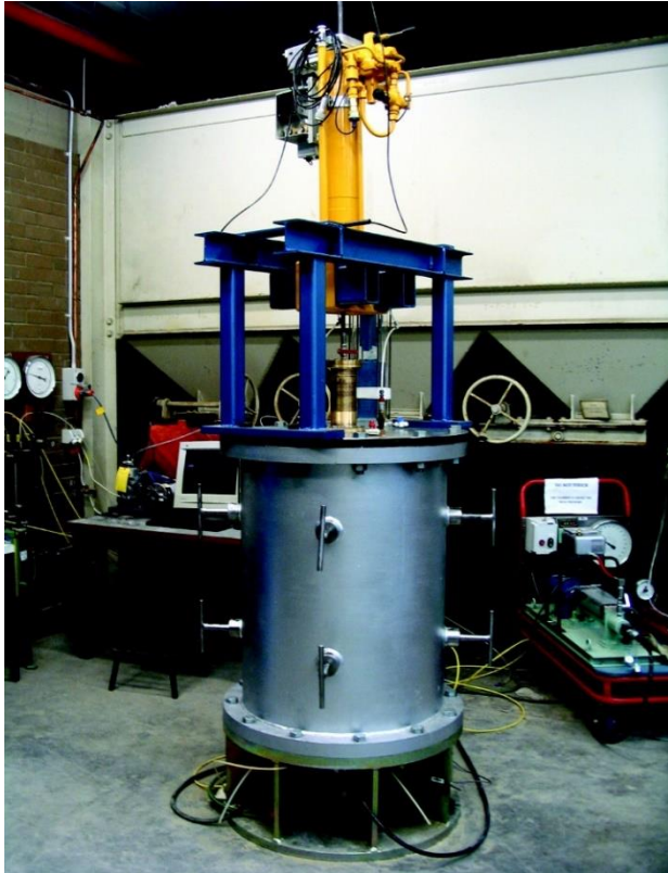
Calibration Chamber in University of New South Wales
